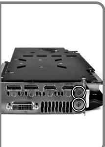
Remove original VGA stock cooler (Remove the screws circled on the diagram. All heat sink assembly screws should be removed)
