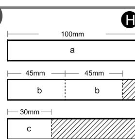
Cut the thermal pads to the dimensions listed and place them on the spots shown on the diagram.
