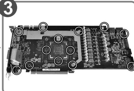
Clean the original thermal compound off the GPU die and remove the screws to detach the backplate. (Carefully detach the original stock cooler after removing all screws securing the cooler to the board)
