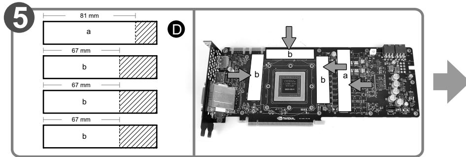
Cut the thermal pads to the dimensions listed and place them on the spots shown on the diagram.
