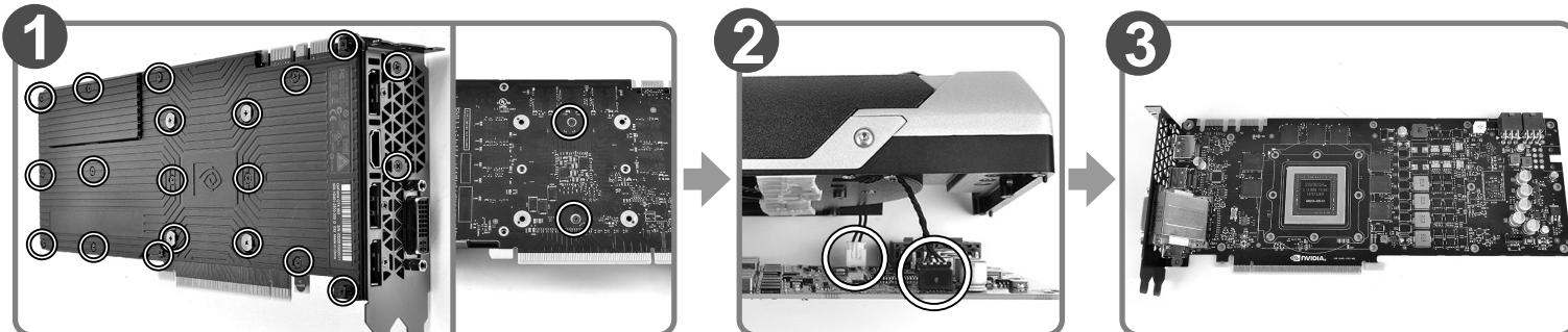
Remove original VGA stock cooler (Remove the screws circled on the diagram. All heat sink assembly screws should be removed)
