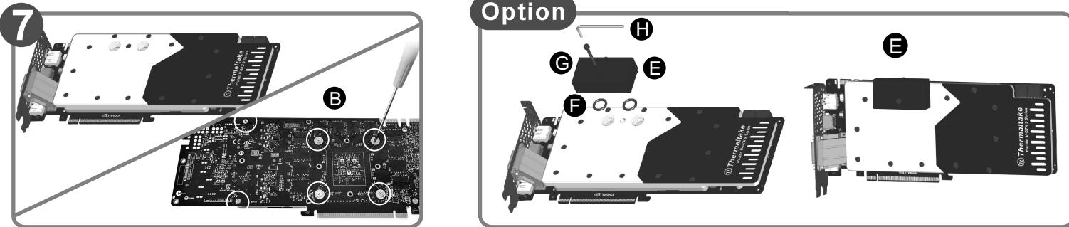
When installing the water block, carefully position the water block with the preinstalled standoffs on the graphics card.
