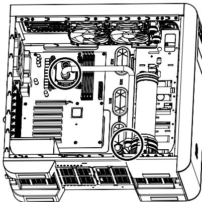
**3** Connect the tubing and check all the fittings are sealed. The loop order: Radiator > Reservoir Inlet
