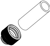
**2** Connect the tubing and check all the fittings are sealed. The loop order: Pump Outlet > Water Block
