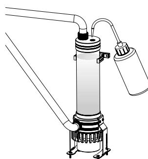
**3** Place your PSU outside of the case and attach it to the pump's 4pin molex connector, turn on the power of PSU and make the rest of the system fills up.
