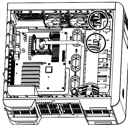
**4** Connect the tubing and check all the fittings are sealed. The loop order: Water Block > Radiator
