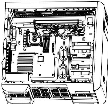
**3** Attach the pump and reservoir into the chosen locations.
