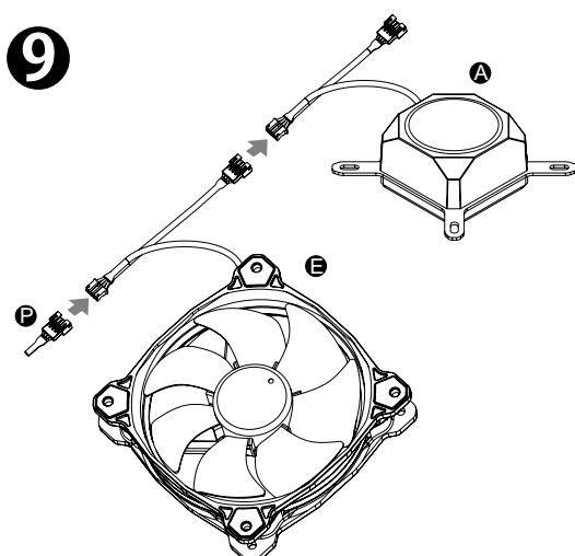
Connect the mainboard sync cable to mainboard.
