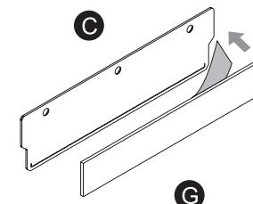
Attach Thermal Pad(G) to the Heat Sink(C)
