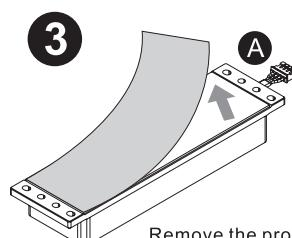
Remove the protective film of Thermal Pad from the Water Block(A).
