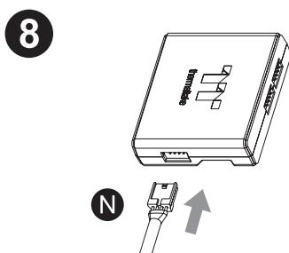
Connect the power cable to the 4pin Molex connector and controller.
