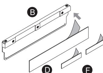
Attach Thermal Pad(D、F) to the Heat Sink(B)
