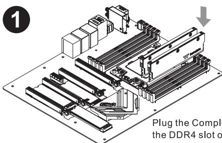
Plug the Complete memory module to the DDR4 slot on the motherboard.
