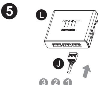
Connect the Waterblock onto the controller.
