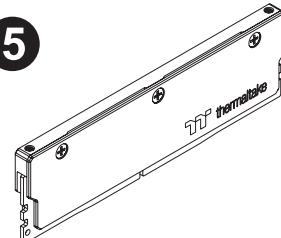
Install the RAMs on Heat Sink(B).
