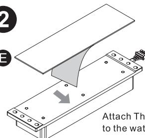
Attach Thermal Pad(E) to the water blcok.
