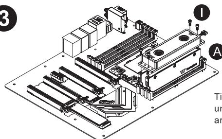
Tighten the Screws(I) until Memory Module are securely attached.
