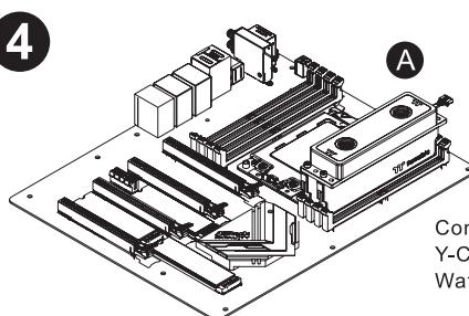
Connect the LED Y-Cable to the Water Block.
