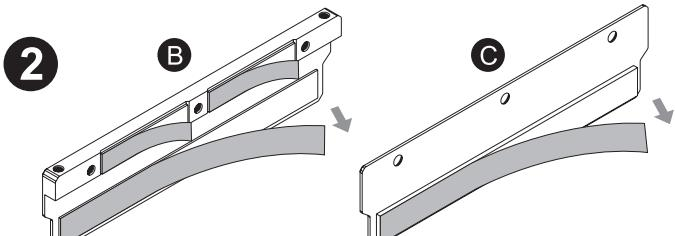
Remove the protective film of Thermal Pad on Heat Sink(C) and Heat Sink(D).
