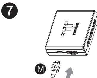
Connect the controller cable onto the motherboard (USB 2.0 9 pin) and controller.
