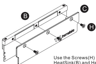
Use the Screws(H) to enclose the HeatSink(B) and HeatSink(C).
