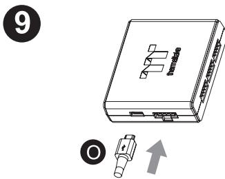
If you want to connect two or more controllers, you can use the bridge cable to connect the controllers.
