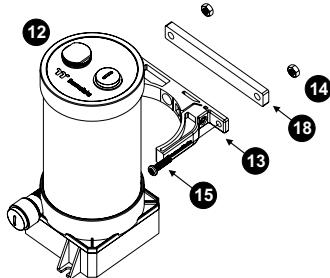
Attach fittings onto the pump and reservoir
