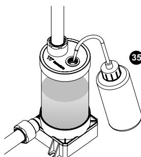
**3** Place your PSU outside of the case and attach it to the pumps 4pin molex connector, turn on the power of PSU and make the rest of the system fills up.
