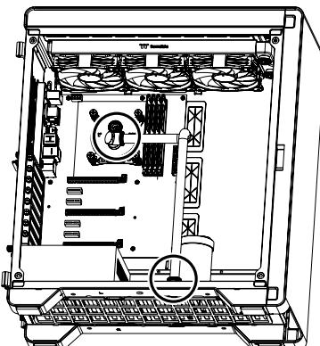
**2** Measure the tube length based on the base part of the fitting, and make (bend) the tubes. The loop order : Water Block > Radiator
