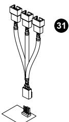
Connect the fan power cable to PWM cable
