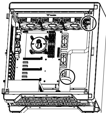
**4** Fit the C-Pro fitting to the tube according to the order in the picture below, Install the tubes and tight the fitting caps.
