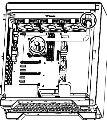
**3** Measure the tube length based on the base part of the fitting, and make (bend) the tubes. The loop order : Radiator > Reservoir inlet
