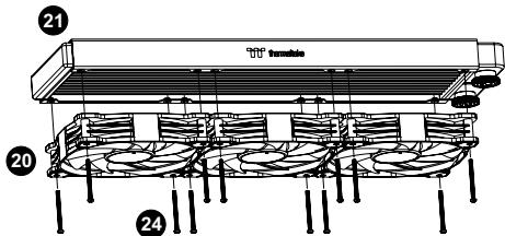
**Connect the fan power cable when the liquid cooling system is completely finished**
