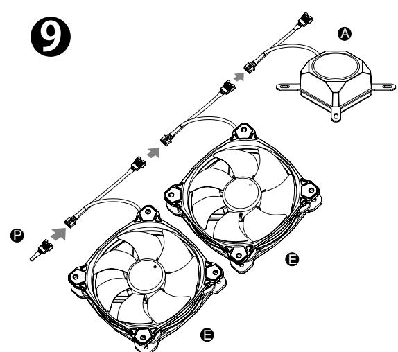
Connect the mainboard sync cable to mainboard.
